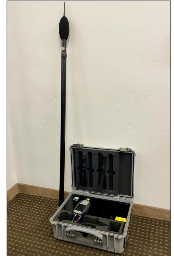
Figure 4. B&K Class I, 2250 Sound Level Meter and associated field equipment.
