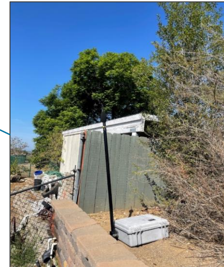
Figure 3. Portable Noise Monitor Set Up
