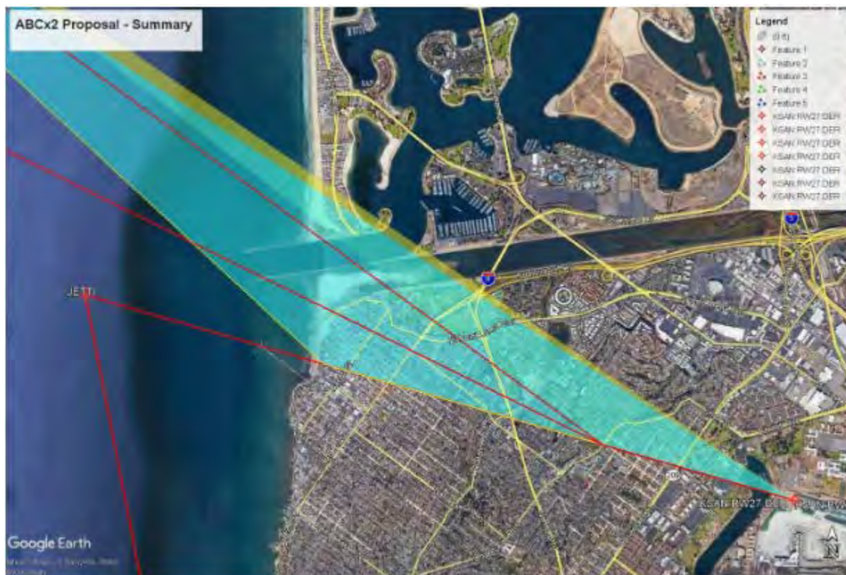
Fig. 9 – ABCx2 Proposed Tracks (Three tracks in red) within the current splay. Blue shaded area includes existing CWARD/PADRZ SIDs and yellow is the additional area covered by the existing ECHHO/MMOTO SIDs.
