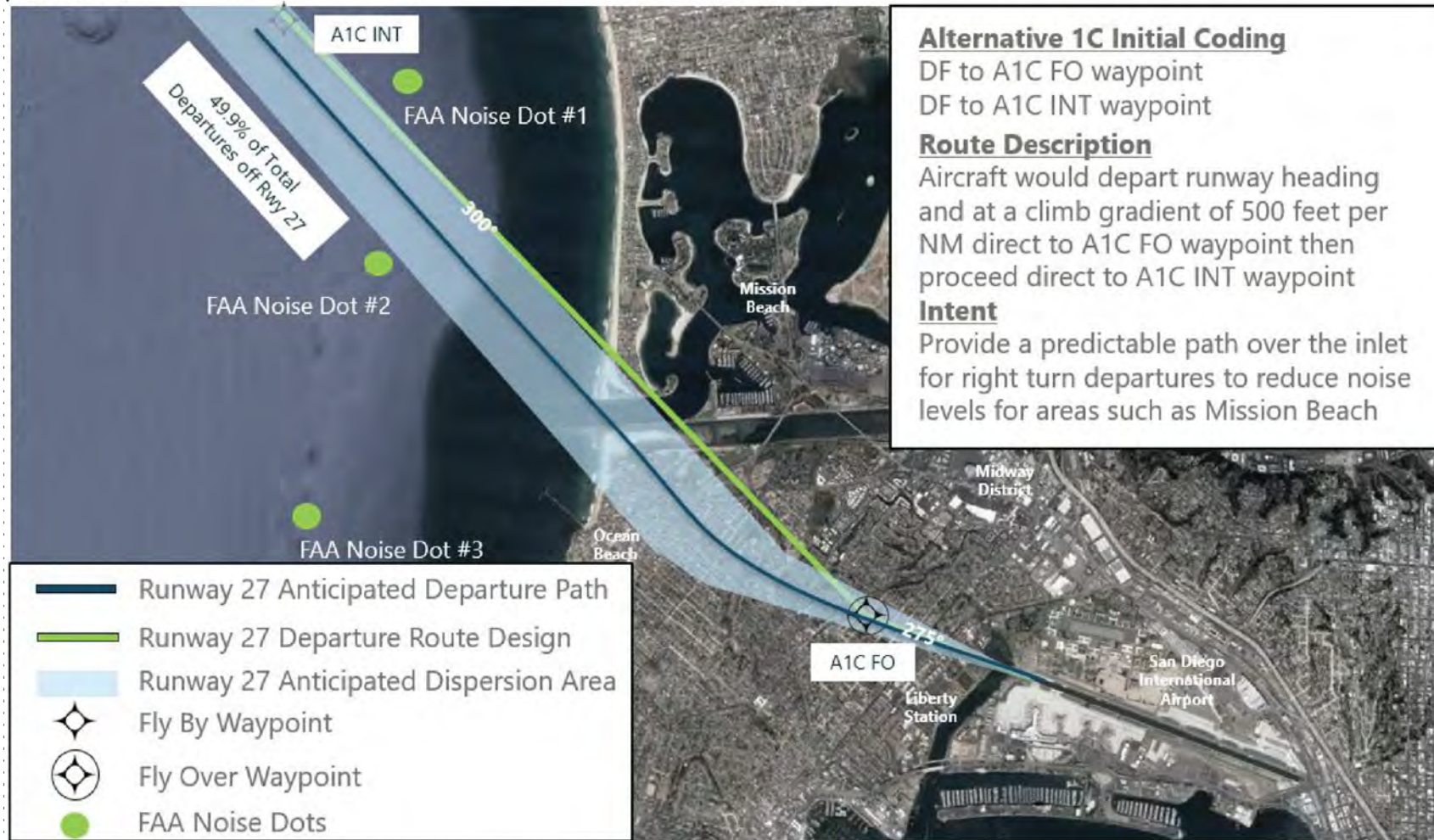
SOURCE: Google, January, 2020 (aerial photo); Ricondo & Associates, Inc., January 2020 (proposed paths and dispersion area).
