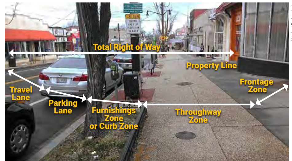
Figure 2-5. In this setting, pedestrian-friendly zones have a relatively high amount of space in the right-of-way relative to the size of the street.
