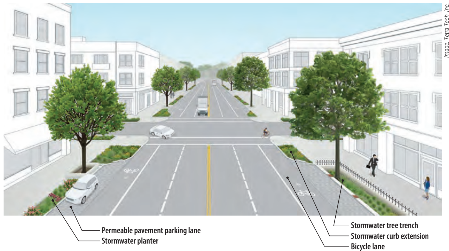
Figure 2-2. A collector road with green infrastructure features in a neighborhood business district.
