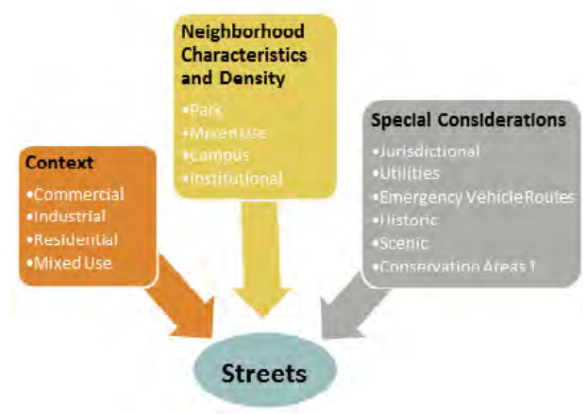
Figure 2-1. Numerous factors must be considered when choosing and siting green infrastructure practices as part of a green street design.
