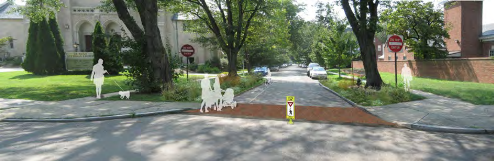
Sketch of green street components such as a permeable pavement crosswalk, curb bump-outs and bioretention applied to a local road.
