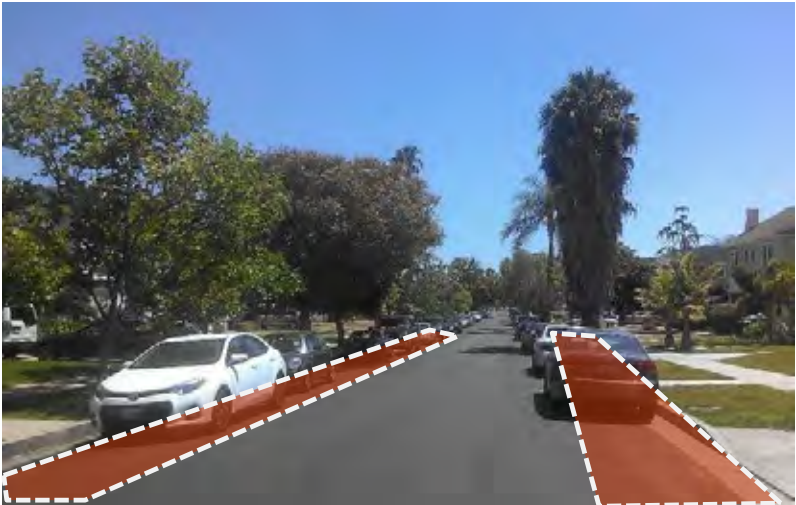
Figure 2-9. Alternative surfaces such as permeable pavement can be used in on-street parking lanes.
