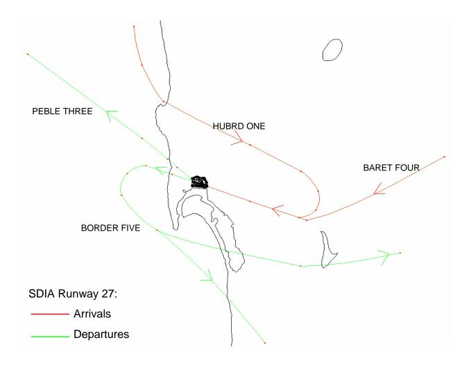
Figure 3: Modeled Flight Tracks at SDIA Runway 27
