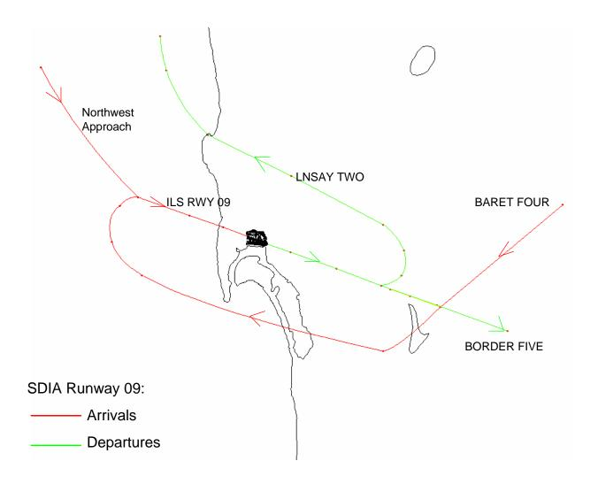
Figure 4: Modeled Flight Tracks at SDIA Runway 09
